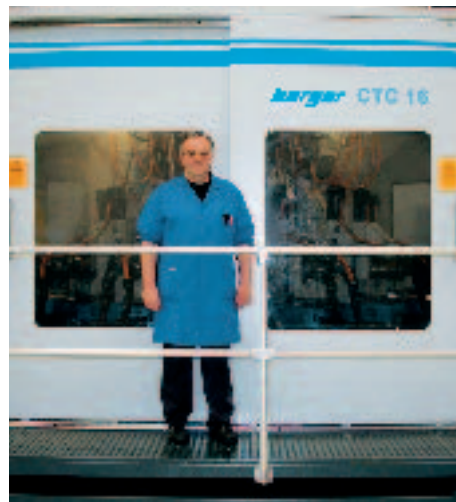
Revolving machine with up to 96 CNC axes
