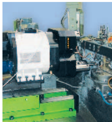
After: Rebuilt machine with drum-type indexing unit and two multiple spindle heads. Cycle time reduced by 42%.
