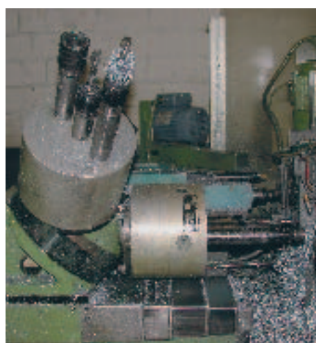
Before: Star-type indexing unit with 2 multiple spindle heads. Cycle time > 19 seconds.
