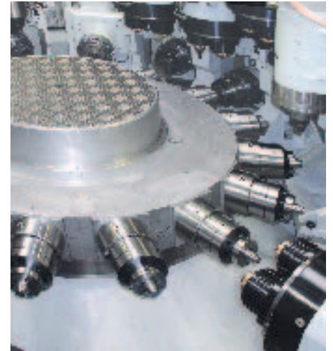
Three-spindle indexing head with HSK 40 interface and two servo drives. Changeover time of less than 1.5 seconds from cut to cut, internal coolant fluid supplied at up to 70 bar, speed of up to 10,000 rpm, also available as receivers for 4 or 5 spindles. Thanks to the compact drum shape, the ancillary stations can also be employed.
