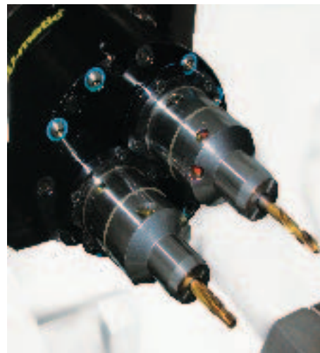
Two-spindle head with HSK 40/50 interface, internal coolant fluid supplied at up to 70 bar, speed of up to 10,000 rpm
